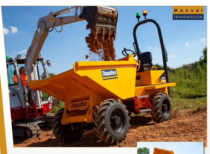
The Thwaites 2 Tonne Front Tip, Stage V dumper is manufactured with contractors and hirers in mind - ensuring operator safety, reducing risk on site and improving performance. Powered by an 18.1 kW 3-cylinder Yanmar engine, delivering 107 Nm max torque for optimum traction and control. This machine is driven by a Manual transmission.
