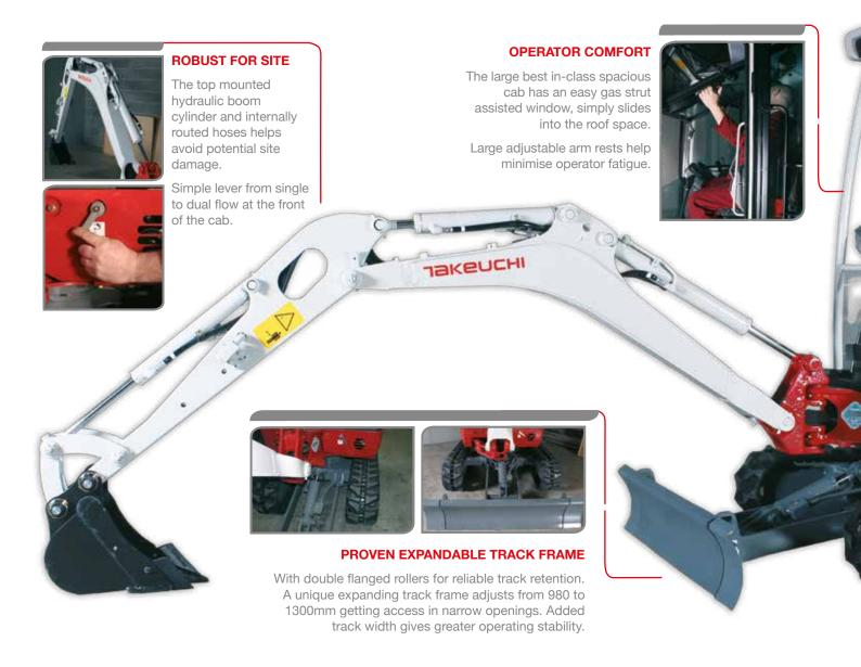
The TB216 is a very well protected mini digger built for the toughest site conditions.
