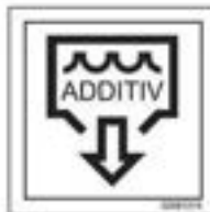
Water tank outlet of additive sprinkling
