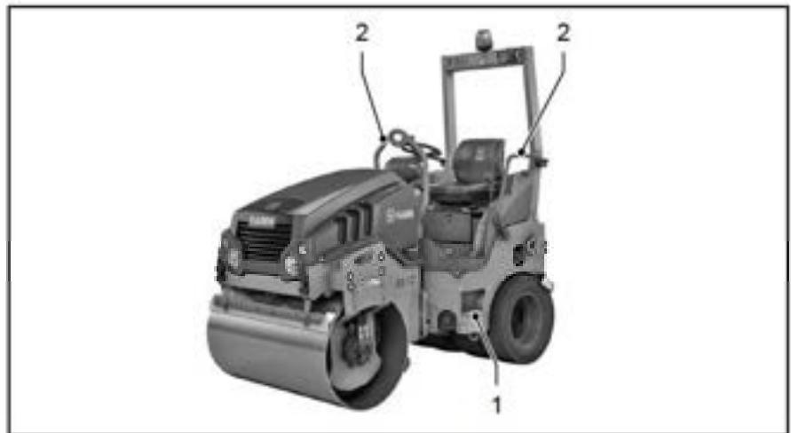
[1] Step to driver's cab [2] Handrail
