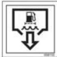
Water sump fuel filter outlet
