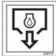
Drain outlet for engine oil
