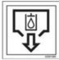
Drain outlet for hydraulic oil tank
