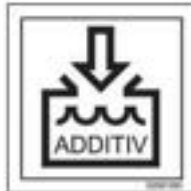
Filling inlet for water tank for additive sprinkling
