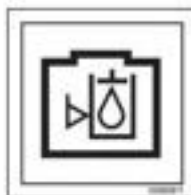
Hydraulic oil fill level
