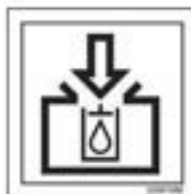
Filling inlet for hydraulic oil tank
