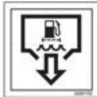
Drain outlet for fuel filter water sump
