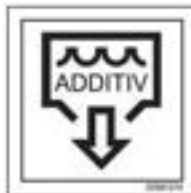
Drain outlet for water tank for additive sprinkling
