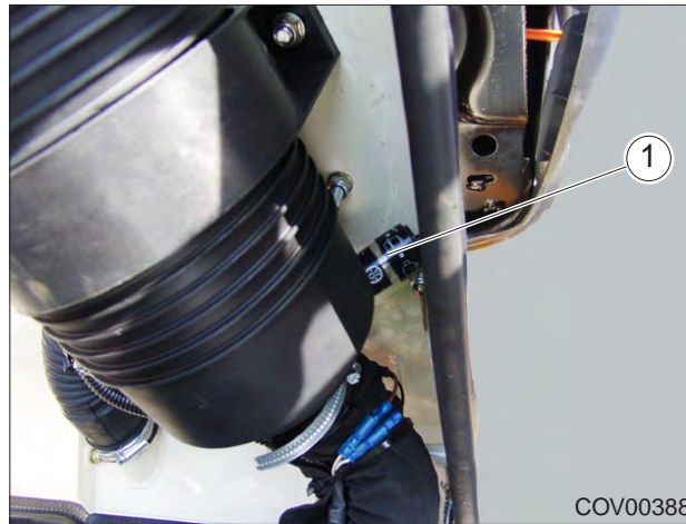
Figure 9.5 Air Cleaner Blockage Indicator.
